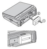
Make sure that the battery pack is not inclined and is locked to the VCR securely.
